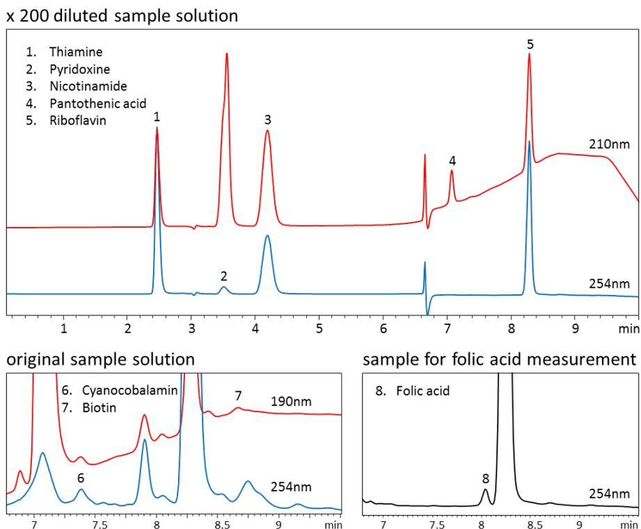
Fig. 4 UV chromatograms of the extract from a commercial multi-vitamin supplement
