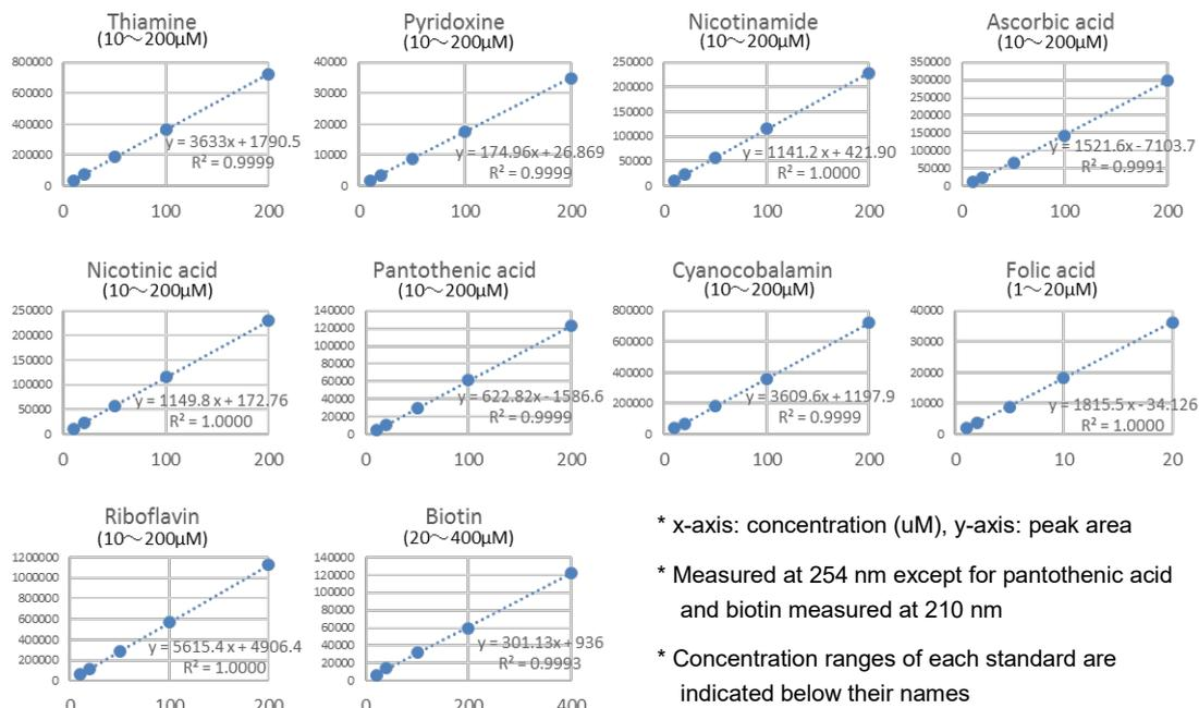
Fig 3. Calibration graphs of ten water-soluble vitamins
